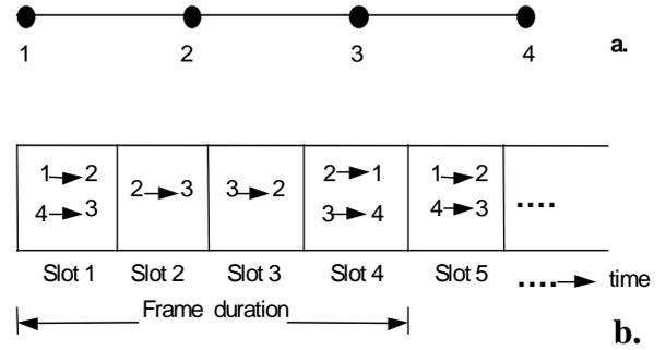
Figure 5: Basic terms used in S-TDMA a. A tandem network of four nodes. b. Schedule of the tandem network. 2→3: node 2 transmits and node 3 receives.
