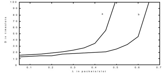
Fig. 7: Packet Delay vs. traffic load. (Network C,  $\sigma = 40m$ ,  $\rho = 3m$ . S-TDMA. a: BS, b: Enhance Scheduling. Network C is similar to Network A minus two radio links: one link between nodes 6 & 7 and second one between nodes 9&10 are both disconnected.
