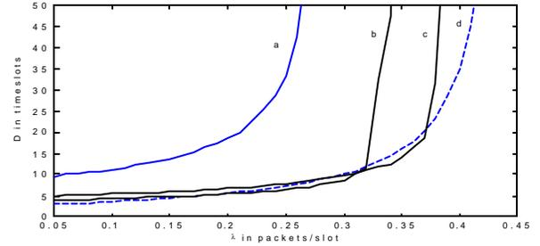
Fig. 4: Packet Delay vs. traffic load (Network B,  $s=40m$ ,  $\rho=3m$ ). S-ALOHA. Strategy II: curve a. Strategy III b:  $k=1.50$ , c:  $k=1.25$ , Strategy I: curve d. The network connectivity is  $\bar{N}=4.2$ .
