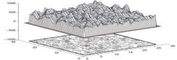
Fig. 1: Plot of terrain realization.  $\mathbf{s}=40$  m,  $\rho=3$  m. Heights vary between 0 and 1200 meters, and the area is  $28 \times 28$  km<sup>2</sup>. (Vertical scale in meters).
