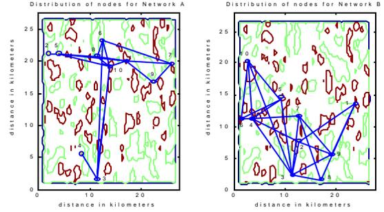
Fig. 2: Typical network realizations in terrain in Fig 1.  $N=10$  nodes. The lines represent the connections among the nodes.
