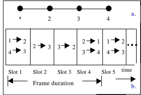
Fig. 5: Basic terms used in S-TDMA a. A linear network of four nodes. b. Schedule of the network.  $2 \rightarrow 3$ : node 2 transmits and node 3 receives.
