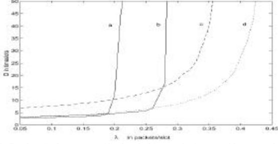
Fig. 3: Packet Delay vs. traffic load (Network A,  $s=40m$ ,  $r=3m$ ). S-ALOHA. Strategy III a:  $k=1.75$ , b:  $k=1.50$ . Strategy II: curve c, Strategy I: curve d. The network connectivity is  $\bar{N}=3.2$ .
